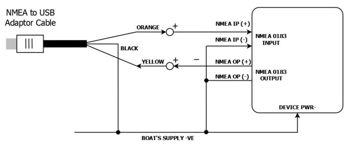
For devices that just have a single positive Input or Output (such as many Garmin or Standard Horizon units) then you should connect it up as shown at the top of the next page. As long as the BLACK wire of the NMEA to USB Adaptor cable is connected to the same DC Supply negative as the device is powered from, then the data will be correctly transmitted and received.
