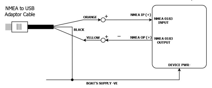
The two previous diagrams show how to wire the cable up for bi-directional communication, if you just want to receive data on to the computer, just wire up the Yellow and Black wires.
